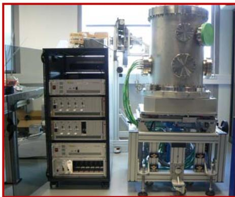
The CASTOR setup (right) and its control and readout electronics (left).
