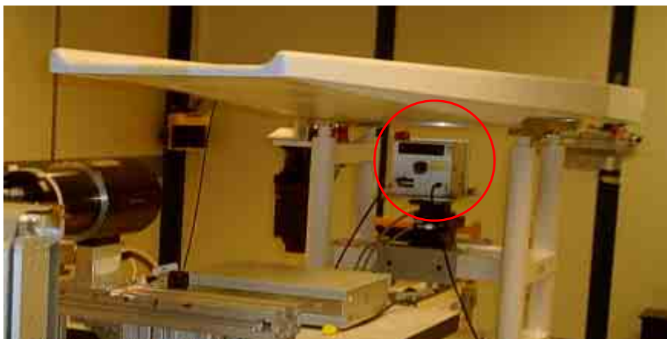
Figure 8. The INMRI-FAC chamber for low energy x-rays at the reference measurement point (inside the red circle) under the patient support shown in figures 5, at SYRMEP beamline.
