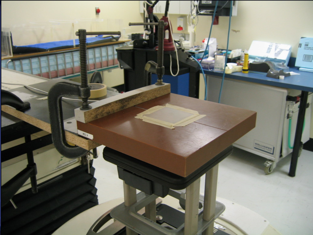
Backscatter setup with aluminum plate covering NACP-02
